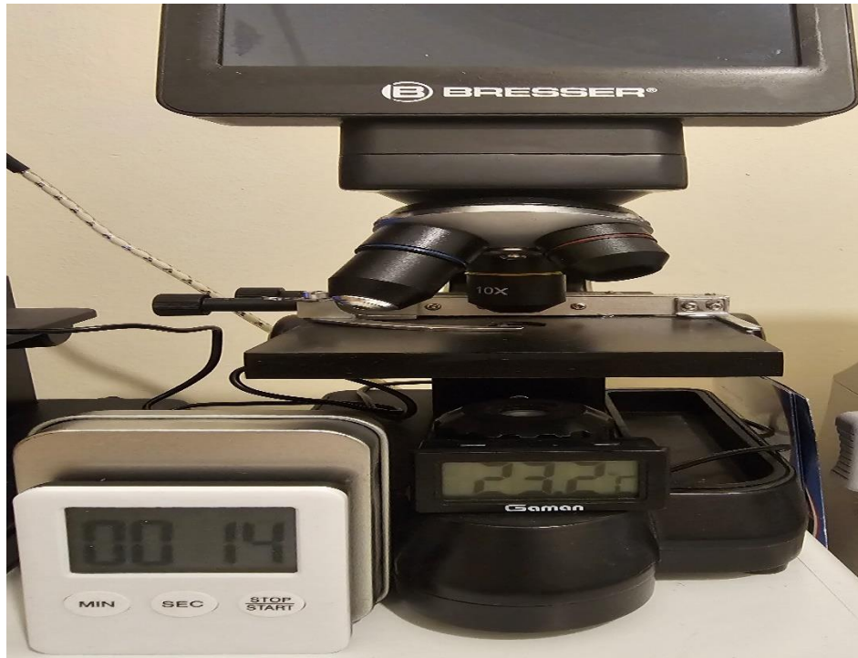
Figure 1 Bresser microscope attached with a thermometer to measure the heat of the slide
