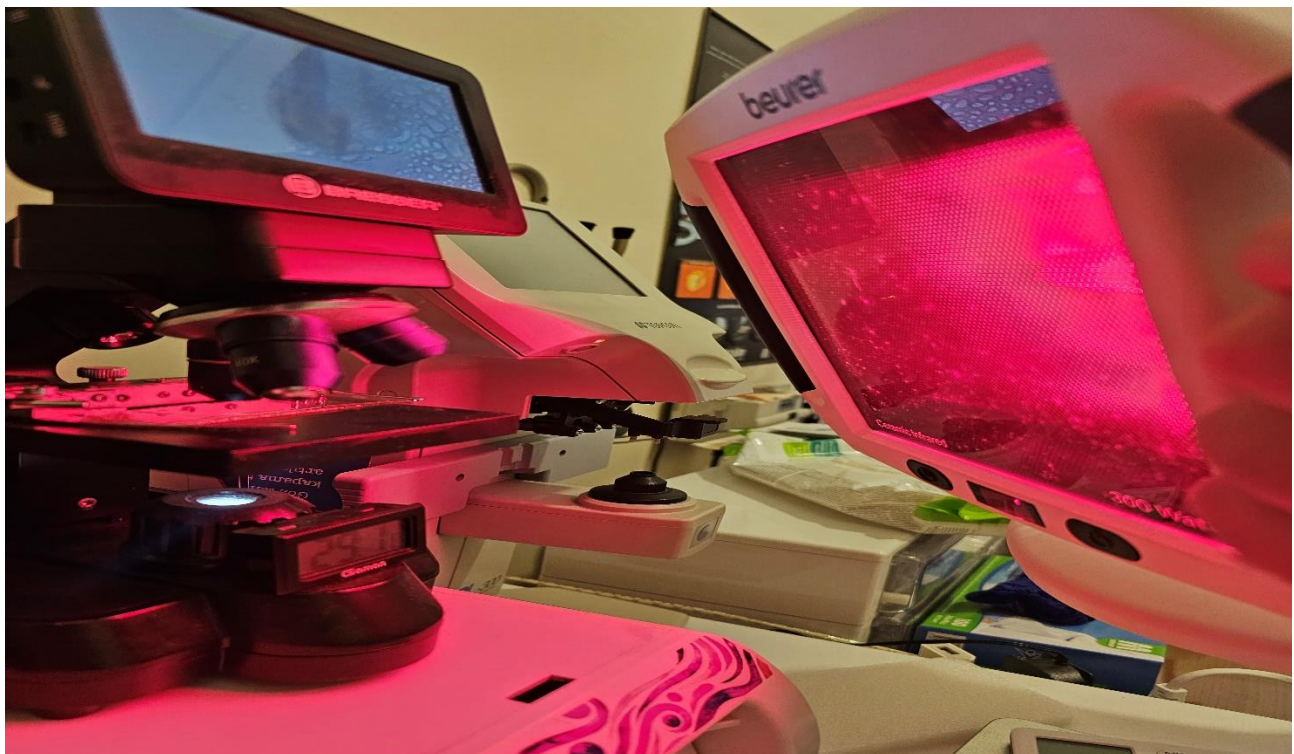
Figure 2 Infrared Heater which is used for heating the slide up to 45°C
