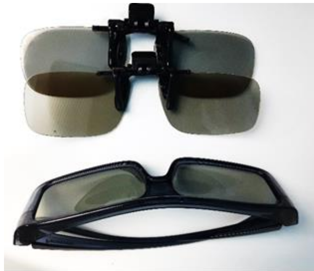
Figure 3: Shows 3D circularly polarized clip-on glasses (above panel) and polarization glasses (lower panel) for use with a 3D monitor
