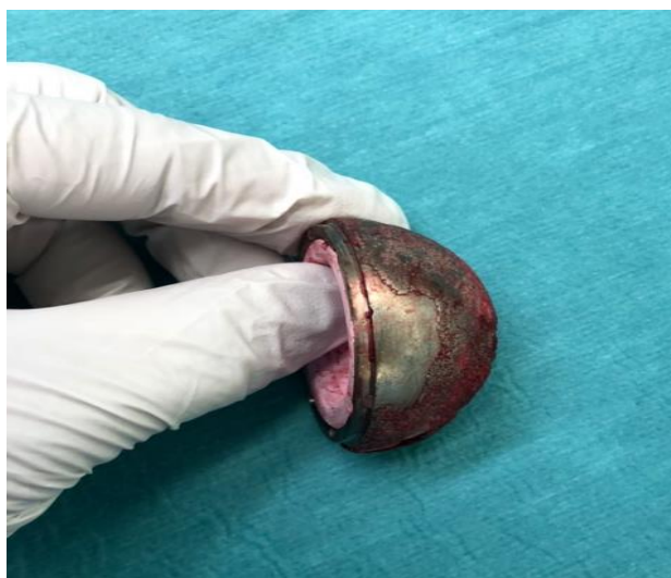
Figure 4. Removed Acetabular Component showing complete loss of surface coating over the exposed area.
