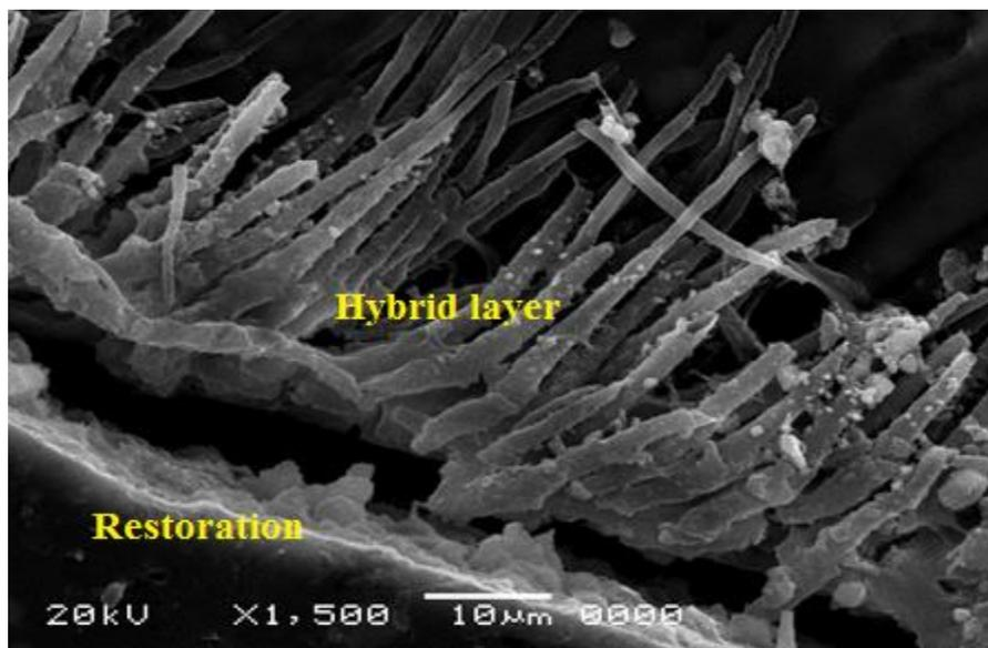
**Figure (6):** Scanning electron photomicrograph for the resin dentin interface (at 1500X) of Kalore at six months storage showing gap at the interface.
