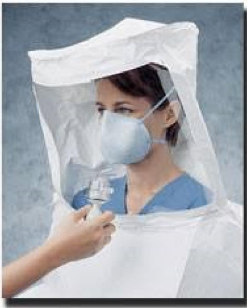
Figure 6 : Fit testing N95 facial mask with qualitative solutions (isoamyl acetate, saccharine, etc.)
