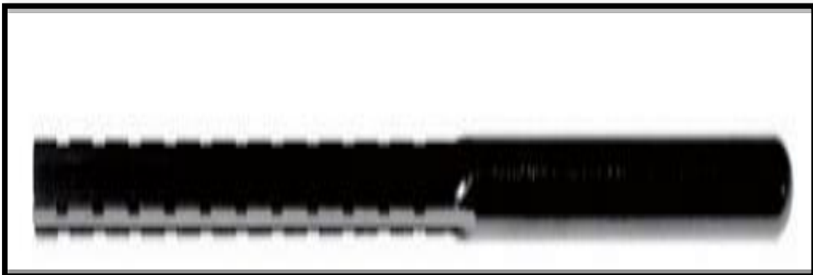
Vertical cutter- prepares a channel for the threaded pin
