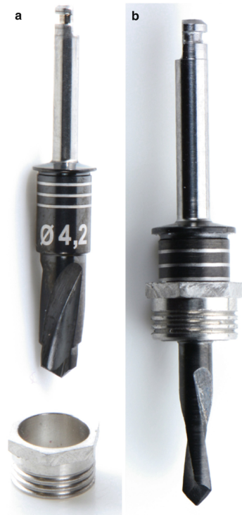
Figure-41: Guided drills with their cutting and guided segments. Half the length of the guided segment must be positioned within the sleeve for the drill to be guided. Therefore, a stepped approach is recommended, starting with initial lengths until reaching desired final depth 41
