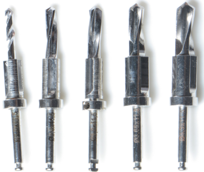
Figure-39: Guided drills design. A cutting portion is followed by a guided segment that corresponds to the inner diameter of the sleeve. the first three drills contain information for a smaller sleeve while the other two adapt to a bigger diameter sleeve, indicating this system has different sleeve sizes for different implant diameters 41
