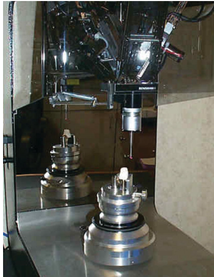
Figure-3: Former contact scanners. Procera® by Nobel Biocare 78
