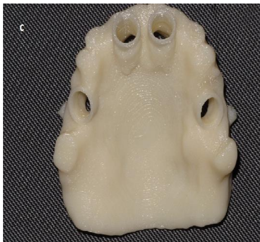
Fig. 3: the computer-generated final design 3D object of the SGT (Left), the 3D printed SGT with fused deposition modeling (FDM) technique of rapid prototyping.
